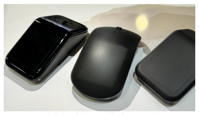
Examples (prototypes) of mice with ambient light panels to power the device.
