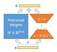
Fig. 34: An illustration of LoRA reparametrizan. Only A and B trained during this process. Courtesy of [142].
